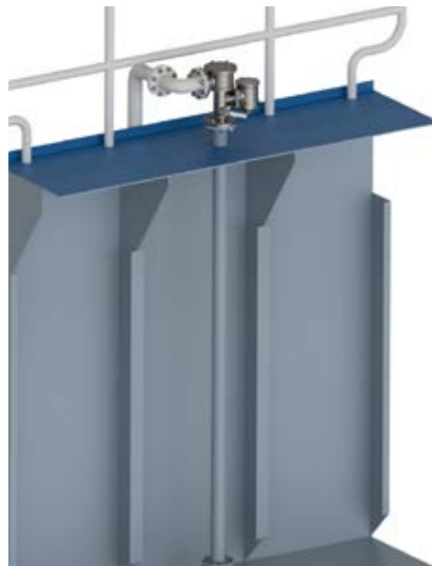
VQ-SUB fitted into a OSV cargo tank vent system
